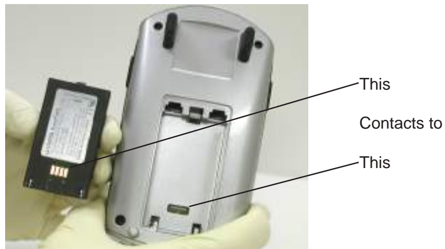
Figure 6.5 Replacing with a Fully Charged Battery
